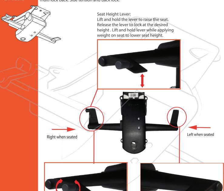
Tilt Tension Control Knob: Turn knob clockwise to tighten the tilt tension and counter clockwise to loosen tilt tension.
